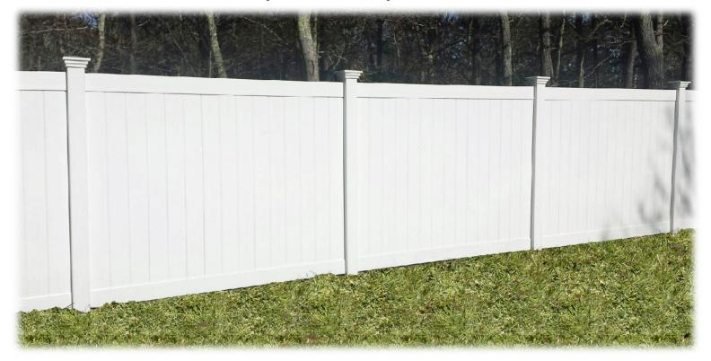
Solid Screen 7/8" x 6" V-Grooved Tongue and Groove Privacy Boards 1 1/2"x5 1/2" Top and Bottom Rails - 5" x 5" (.135" Wall ) Posts
